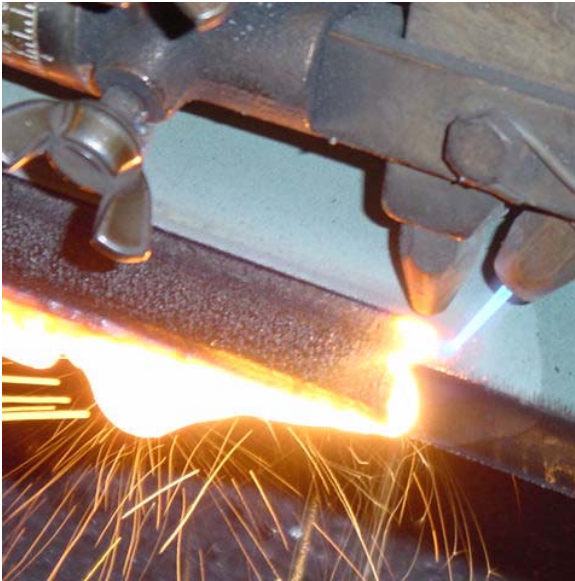
45 degree bevel cut – Coated mild steel plate in Tsuneshi Shipyard, Japan.
