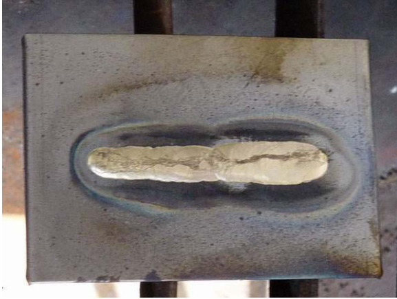
HydroBrazed – Bronze filler on 1.2mm mild steel base metal. No flux residue, clean appearance
