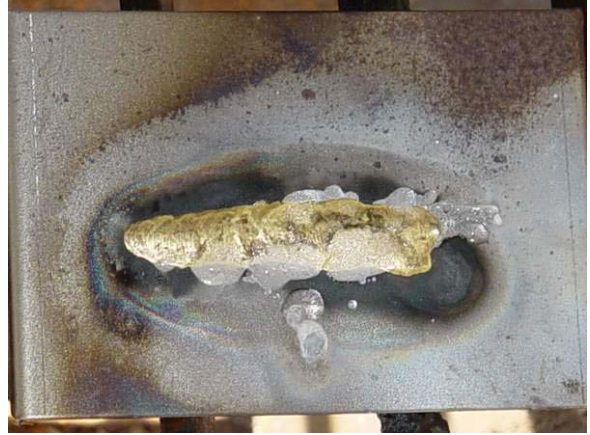
Acetylene Brazed – Bronze filler on 1.2mm mild steel base metal. Note hard flux residue & large oxidized area
